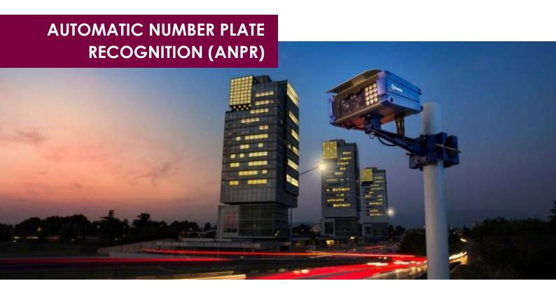
ANPR Also called License Plate Recognition (LPR) is a mass surveillance method that uses Optical Character Recognition (OCR) on images to read vehicle registration plates.
